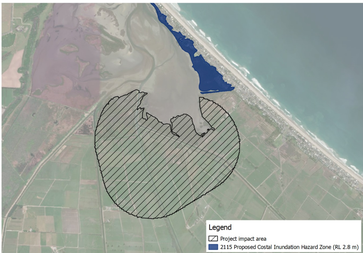
Figure A3.3a. Proposed Coastal Inundation Zone (CHZ) for the year of 2115 (Tonkin & Taylor, 2015).
