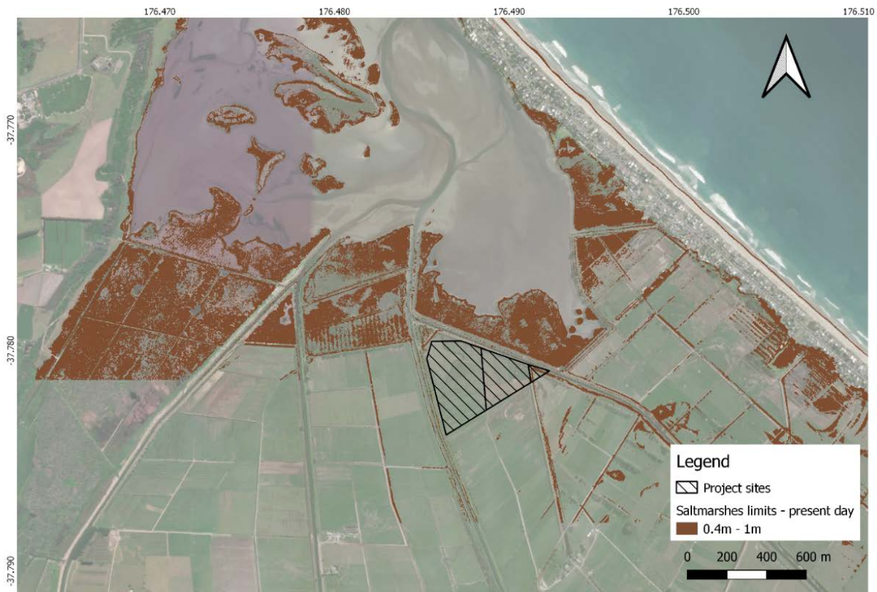
Figure A6.2.3c: The salt marsh habitat zone (SMHZ, reddish brown areas in between salt marsh limits) in relation to the Pukehina/ Waihi Estuary project site. The SMHZ is mapped using a simple approach based on elevation data for the present-day (top plot) and '100-year' (bottom plot) scenarios used in our study.
