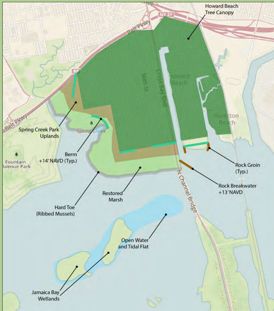
Figure 5-2 Alternative 1: Natural Infrastructure (Shoreline)
